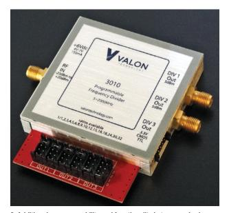
2. Additional programmability and functionality in turn required a larger package for this analog/digital frequency divider. (Courtesy of Valon Technology)
