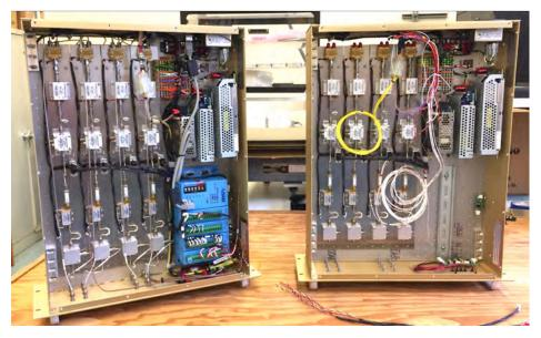
Figure 21. IF processor units under construction. Four IF and baseband paths are visible on the left side of the units. DC power supplies are above the blue monitor and control unit.
