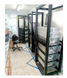
Figure 24. VLBI trailer with Mark-6 recorders mounted in racks.
