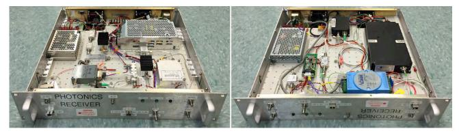
Figure 5. LO photonics receiver assembly. Top view of DC power supplies and RF components, includes round trip phase monitor hardware.
